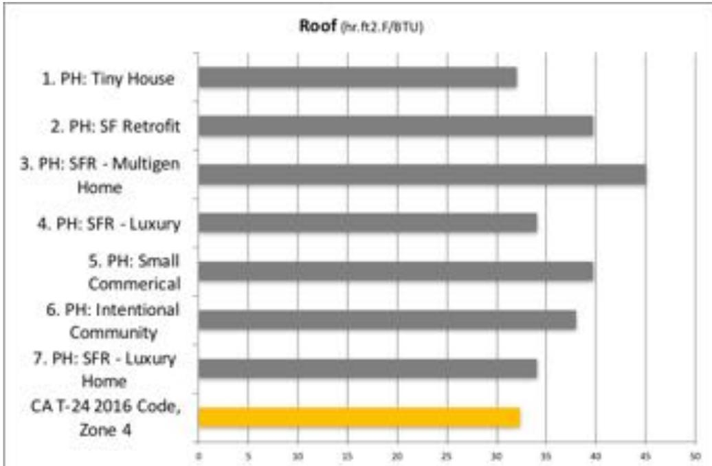
Figure 6. Roof insulation levels shown as 'effective.' (See note in Fig.5)
