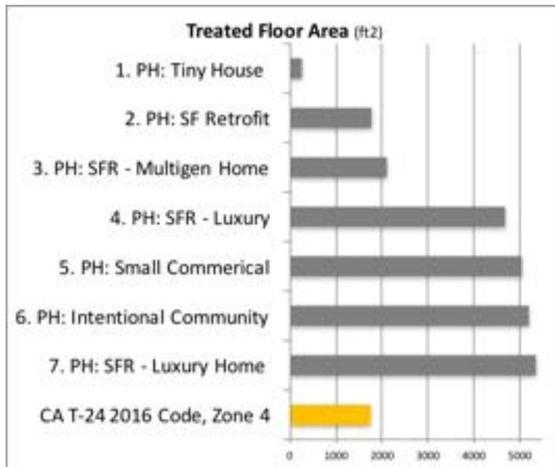
Figure 4 (above): Treated floor area (interior conditioned space) of buildings in Palo Alto's Passive House Cluster plus CA T-24 house based on Palo Alto average house size, reduced by 15% for fair approximation.
