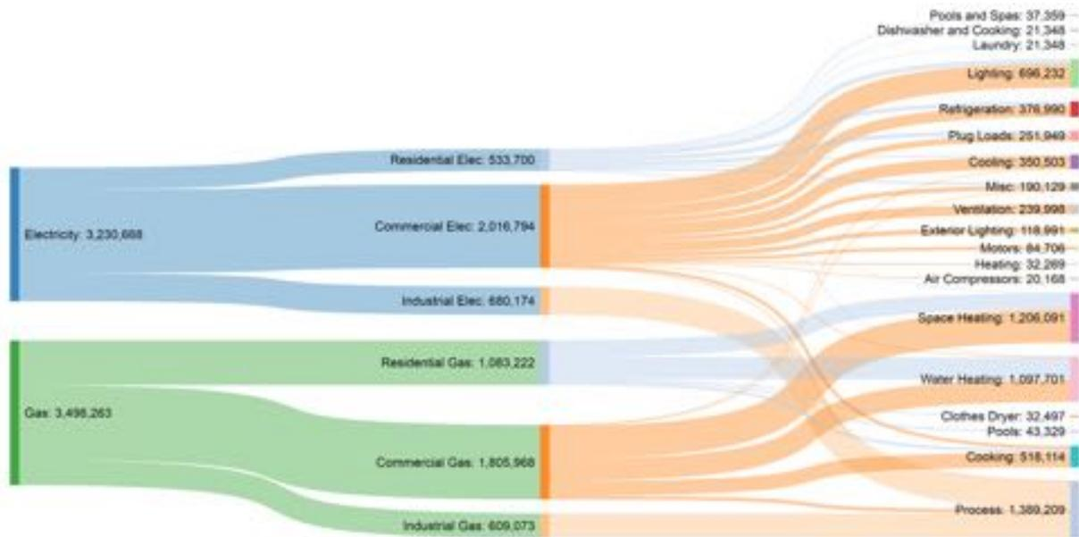
Figure 1. 2016 Palo Alto Building Energy Use Breakdown, disaggregated by type, source and end use. Source: Residential Appliance State Survey (RASS) and California Commercial End Use Survey (CEUS.) Graphic use by kind permission from DNV-GL.
