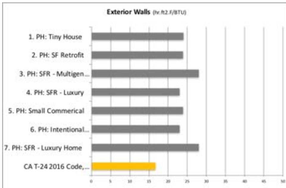
Figure 5 (above): Wall assembly insulation values all include a framing factor reduction and are shown as 'effective,' as opposed to 'nominal.' (eg. R-19 'nominal' - 15% ff = R-16 effective.)
